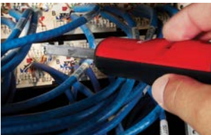
Extended Reach Punchdown Blade
